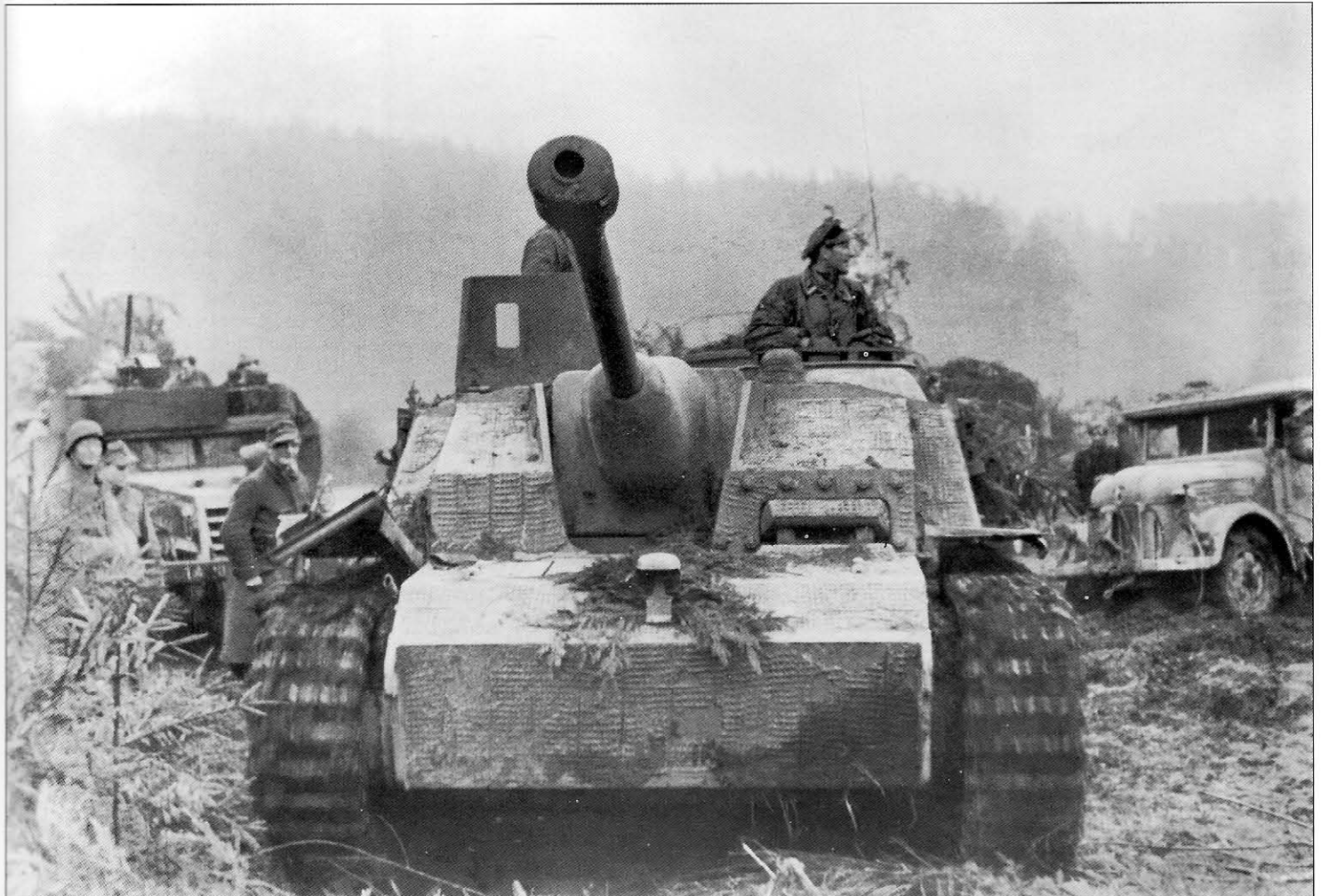
This Sturmgeschütz III Ausf.G of an unidentified SS unit was one of those built by Alkett and features their unique waffle pattern Zimmerit coating. It has been fitted with the 'Topfblende' mantlet, often referred to as a 'Saukopf', and a single 80mm armor plate on the right side of the upper hull identifiable by the absence of the bolts used to attach the additional 30mm armor plates. It was assigned to either 2. or 9.SS-Panzer-Division which both were equipped with two companies of StuG.III/IV in their II.Abteilung. On the right can be seen a Steyr 1500A/01 personnel car and on the left a captured U.S. M2A1 or M3A1 half-track displaying the 1st Army bumper code.
