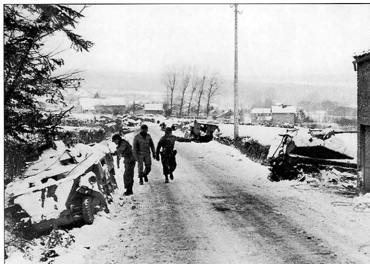
Sd.Kfz.250 half-tracks of 116.Panzer-Division litter the roadside in Amonines after being destroyed by Task Force Orr of 3rd Armored Division. The two half-tracks on the left are 'Neue' production vehicles while the one on the right is an 'Alte' production and is quite unusual in that it has been fitted with a 2cm autocannon.
