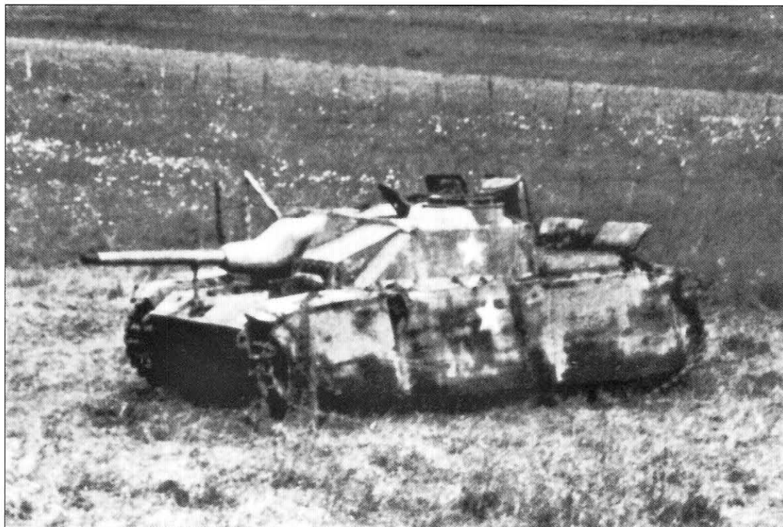
An attempt to disguise the five StuG.III Ausf.G of Hauptmann Scherff's Kampfgruppe Y was made by adding different side skirts and sheet metal on the engine deck but the effort was in vain as they did not resemble anything in use by the U.S. Army. At best, they probably just caused confusion. They carried bumper codes for C Company, 81st Tank Battalion, 5th Armored Division, which was not even in the Ardennes at the time. This one had the number C 5 and was abandoned between Baugez and Géromont.
