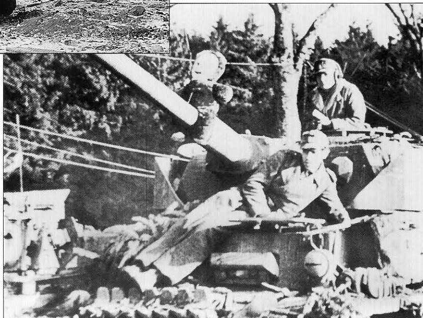
Another photo of the same Panther taken some time later having sustained some additional damage and after the Pz.Kpfw.IV Ausf.J had been moved to clear the roadway. The Flammentöter vertical exhaust can now be clearly seen on the rear of the Pz.KPfw.IV.
