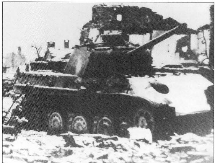
Another of Kampfgruppe Peiper's Panthers abandoned in La Gleize. This one is one of twenty Panthers produced by M.A.N. in late September 1944 equipped with experimental steel tired roadwheels the same as used on the Tiger I and Tiger II. It had the tactical number '221' painted on the side of the turret in black with a stenciled white outline.
