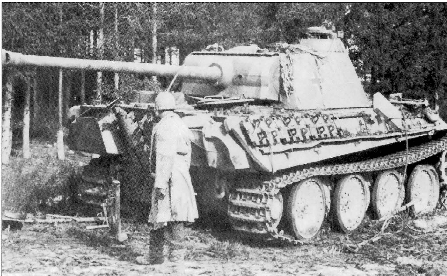
This late production Panther Ausf.G, possibly from the same unit as the previous one, is also fitted with the chin mantlet and raised fan cover but still retains the earlier exhaust pipes and earlier idler. Unusually, it has a Balkenkreuz painted on the side of the turret along with the three digit tactical number '302' in a white stenciled outline.
