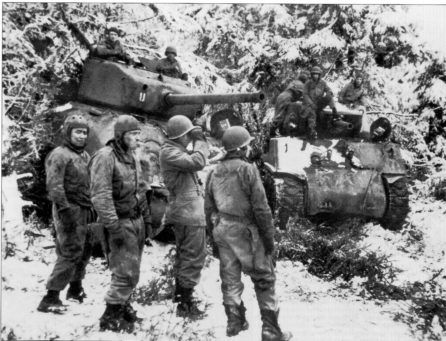
Tank crews from the 3rd Armored Division take a cigarette break at the edge of a forest. The tanks are a Sherman M4A1(76)W and an M4A3E2 'Jumbo' up-armored assault Sherman armed with a 75mm gun. By this time the 'Bulge' was slowly being reduced.
