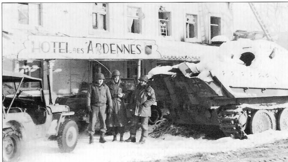
This burned out Panther Ausf.G from 1.SS-Panzer-Division was knocked out near the crossroads at Baugnez. The tactical number, '111', can be faintly seen on the side of the turret. It was produced in late September 1944, after the discontinuation of Zimmerit and the introduction of the reinforced chin gun mantlet but before the larger diameter self-cleaning idler was introduced. Note the unusual location of the Balkenkreuz on the side of the hull just in front of the spare track links.
