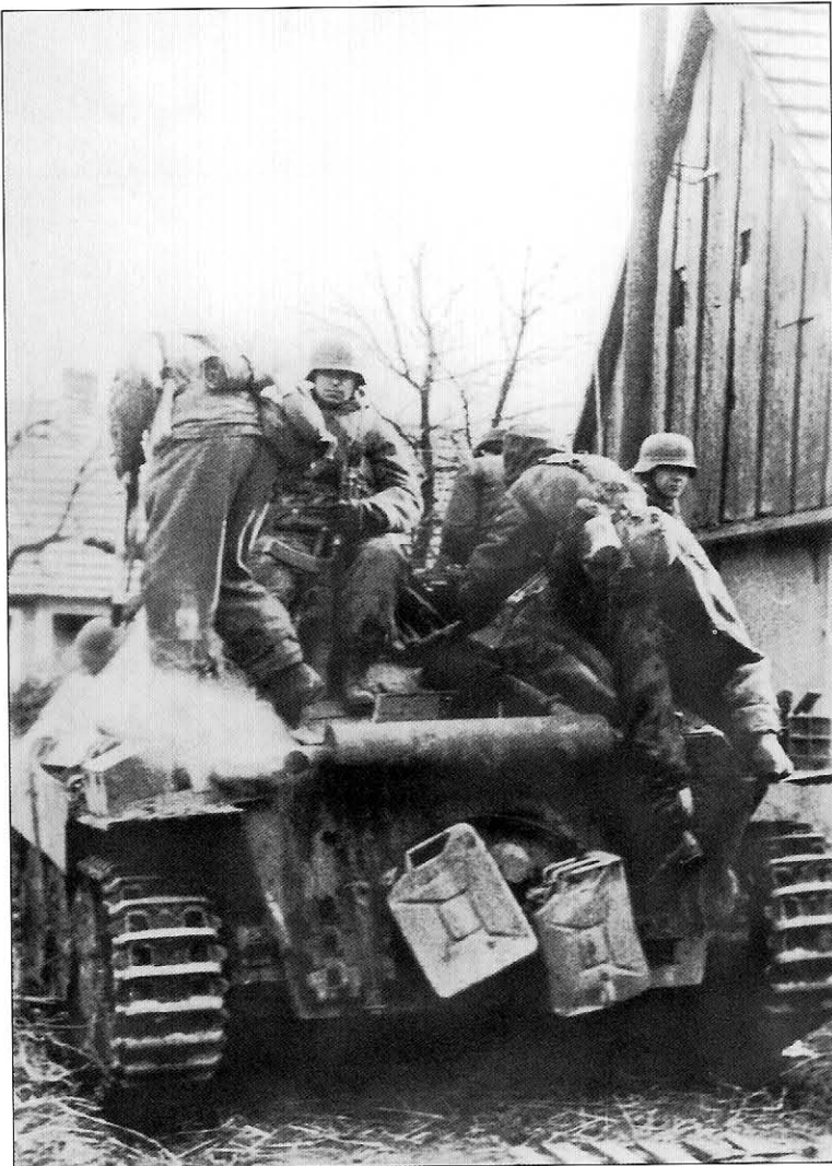
Panzer-Grenadiers climb aboard a Jagdpanzer 38(t) Hetzer. The Hetzer primarily equipped the anti-tank battalions of the infantry and Volks-Grenadier-Divisions to provide armored support. This one is a mid-production version built sometime before October 1944 when the Flammvernichter exhaust was introduced. Two of the grenadiers are armed with MP44 assault rifles.
