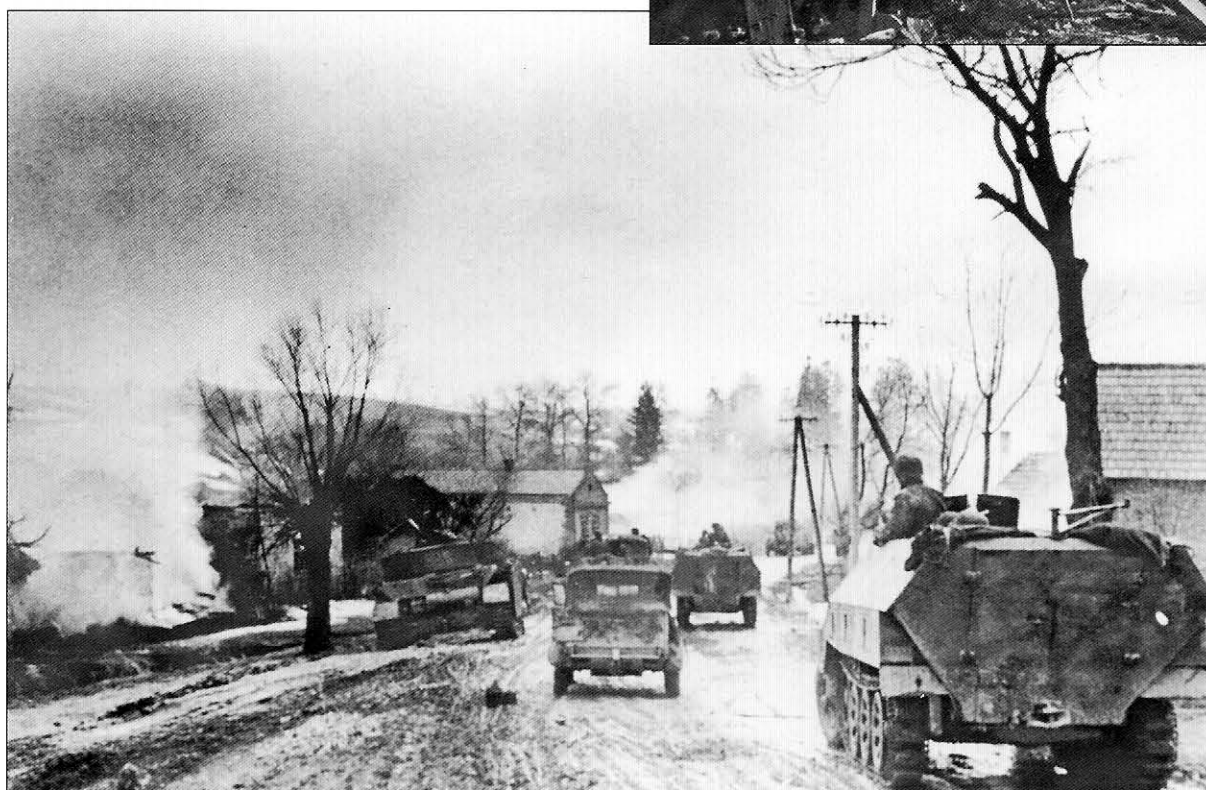
A column of SS-Panzer-Grenadiers pass through a burning Belgian village in their Sd.Kfz.251 Ausf.D half-tracks. On the original photograph, the SS registration plate is faintly visible on the nearest vehicle. The lead half-track is fitted with a star antenna on the left side indicating it is a command vehicle. To the left, a Pz.Kpfw.IV Ausf.H can be seen at the side of the road.
