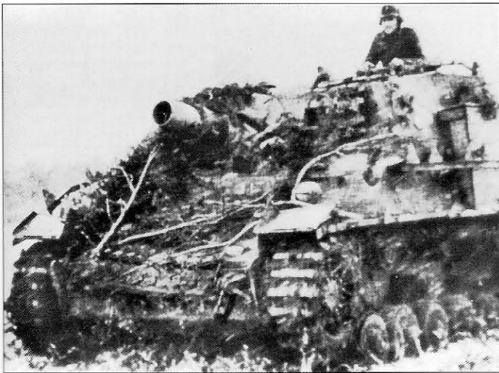
A heavily camouflaged Sturmpanzer IV Brummbar of Sturmpanzer-Abteilung 217 moves into position in support of 12.Volk-Grenadier-Division during its assault on Dom Butgenbach on 22 December. It is a late production vehicle fitted with resilient steel roadwheels and covered with Zimmerit. Markings appear to have been limited to the standard white outlined black Balkenkreuz on the sides of the fighting compartment and front of the driver's plate.
