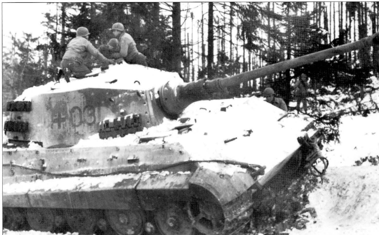
A Tiger II from the battalion headquarters of s.Pz.Abt.506 sits abandoned on the road near Villers-la-Bonne-Eau. It is painted in the factory applied hard edge camouflage scheme of green and dark yellow over the red primer base. Small spots of color have been added to the base colors to complete the 'ambush' pattern. The tactical number '03' appears to be painted in solid black in front of the standard Balkenkreuz.
