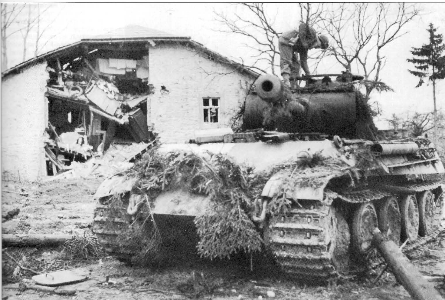
American soldiers from the 75th Infantry Division inspect a knocked out Panther Ausf.G from 2.SS-Panzer-Division in Grandmenil in late December 1944. It is a late production vehicle completed in October 1944 and is fitted with the raised fan cover for the crew compartment heater. In August 1944, jettisonable driver and radio operator hatches began to be installed and one can be seen laying on the ground to the left.
